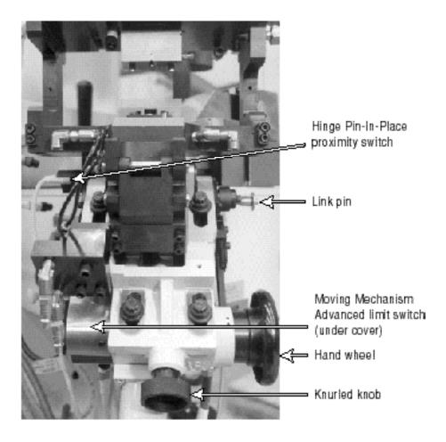
Moving mechanism and limit switch
