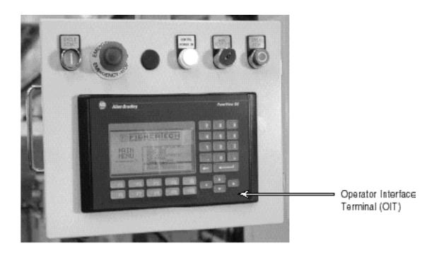
The control pendant, suspended from the pendant arm, houses the push buttons, indicating lights and selector switches as well as the Operator Interface Terminal. Note that individual control devices may vary depending on the termination or assemblies being produced and the operating sequence.
