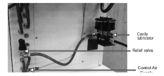
A positive feed lubricator is used to lubricate the tooling. A detailed instruction sheet can be found in Section J: Vendor Supplied Specifications and Maintenance Bulletins. Refer to this instruction sheet for a detailed description of how the lubricator works and how to overhaul the unit.
